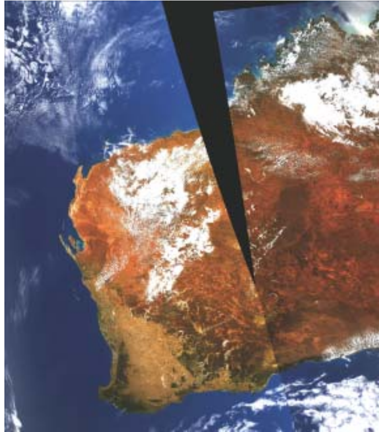
Figure 3: MODIS data after atmospheric correction (applied to land pixels only). The join between the two orbits is clearly visible in the lower right of the image.
