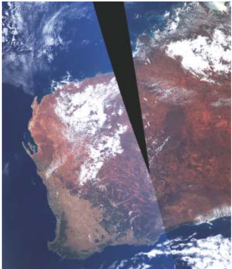
Figure 2: The MODIS data of Figure 1 after radiometric and geometric calibration. The image is bluish and has low contrast due to the scattering and absorption of light by the atmosphere.
