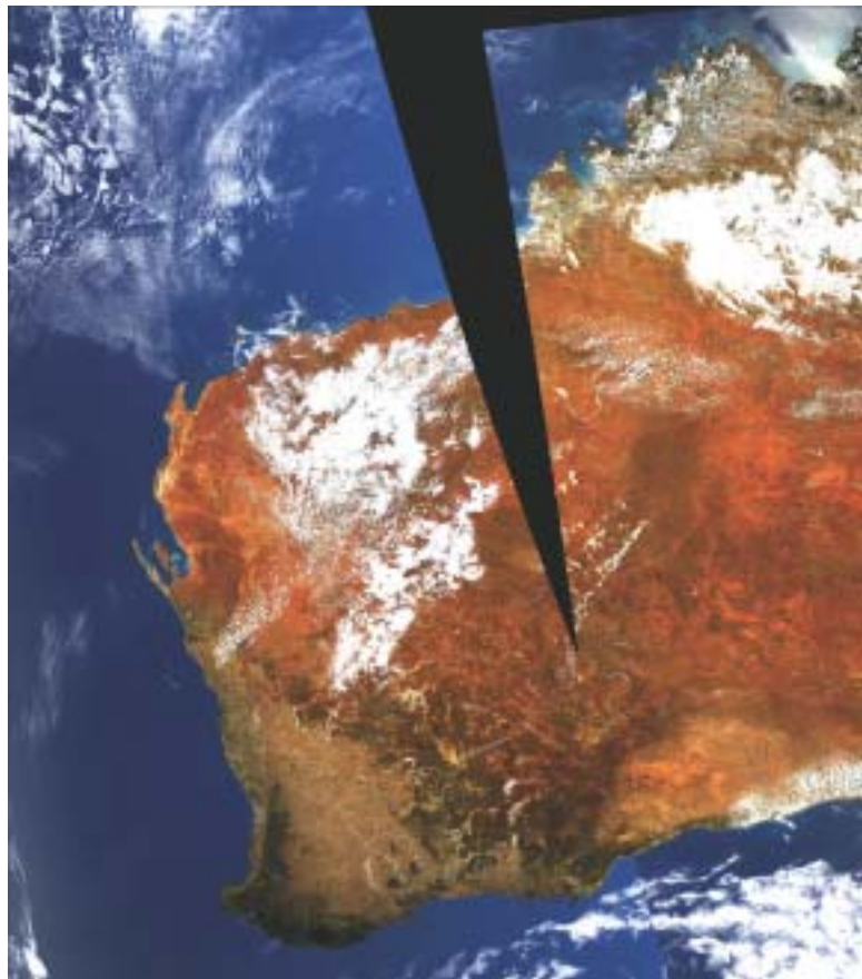
Figure 4: MODIS atmospherically and observation-geometry corrected reflectances (corrections applied to land pixels only).
